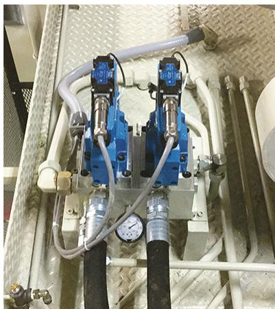
Eurotherm's shoot-and-fill feature synchronizes the filling and emptying of the two hydraulically driven accumulators on a dual-head industrial blow molding unit.
